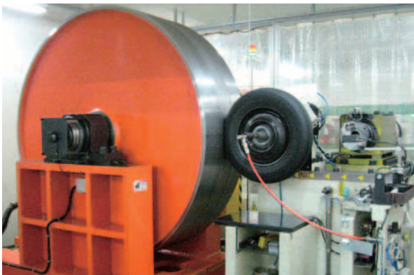
Tire Rolling Resistance Test Equipment
