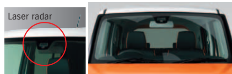
Because the laser radar is located in the operation range of wipers, the radar is activated also in rainy weather. *It may not work when dirt on the windshield cannot be removed due to deterioration of the wiper blade or weather is terrible.
