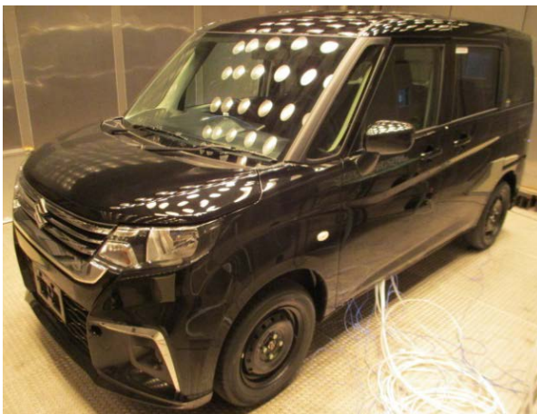
VOC measurement in the cabin (New Solio)
