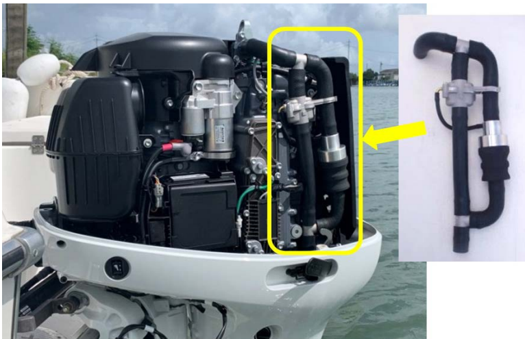
Outboard motor installed with Micro-Plastic Collecting Device
