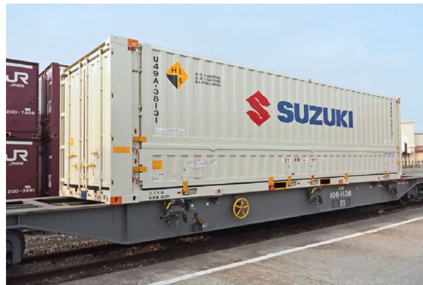
31 ft container for rail transportation
