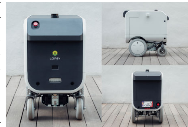
Prototype of autonomous delivery robot using motorized wheelchair base
