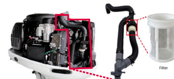
Outboard motor installed with the Micro-Plastic Collecting Device
