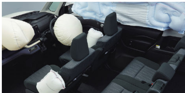
Image of car interior during airbag deployment (model: Solio)
